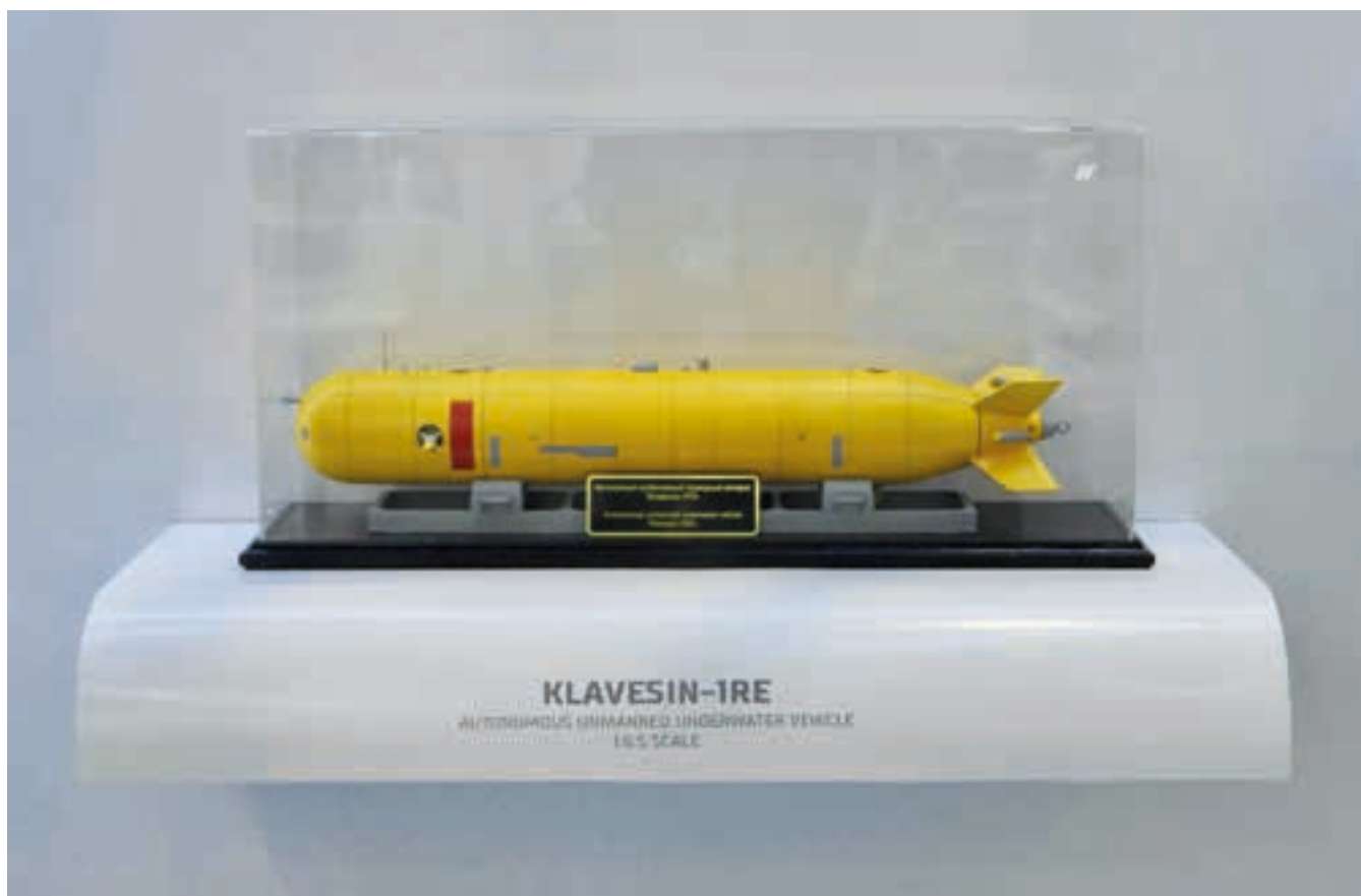
The vehicle's specifications include an operational depth of up to 6000 meters and a range of 280 kilometers (photo: Yury Laskin)
