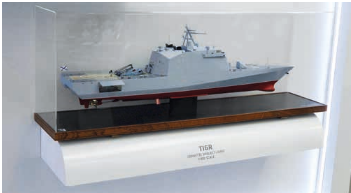
The Tigr can achieve speeds of up to 27 knots and has a range of 3,800 nautical miles at a cruising speed of 14 knots (photo: Yury Laskin)
