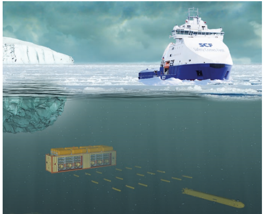
Rubin is currently developing a concept design of a group of AUUVs for marine geophysical exploration to ensure seismic survey (pic.: CDB ME «Rubin»)
